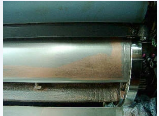
Example of repaired corrosion damage on a blanked cylinder
